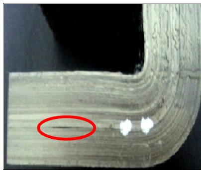
2) Minor gap on top & bottom Surface
